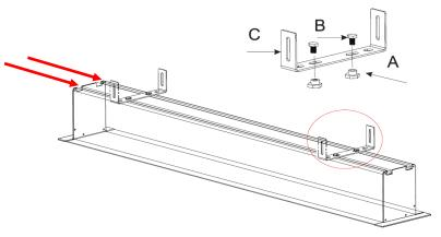
3. Place the Suspension Bar (D) on the Hanging Bracket (C) and align with the hole as shown below. Secure the Suspension Bar (D) with the Hex Screw (B), Washer (E) and the Hex Nut (F). Install the Suspension Bars (D) to your ceiling according to their distance.
