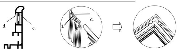
Step 5: Secure the elbow joints by fastening them with M4x7 screws (g), 4 at each corner.
