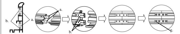
**Step 4:** Connect the *elbow joints* (*c/d*) to the top and bottom sections of the vertical frame. Once inserted, connect the vertical sections to the horizontal frame sections. Make sure all holes are in alignment and the frame pieces are flush (no gaps). They should form perfect right angles.
