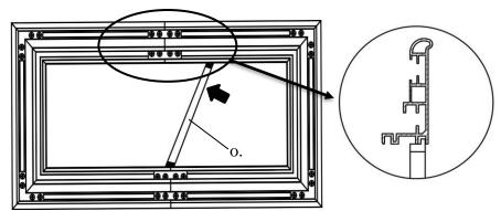
**Step 9:** 1. Insert iron eyelet through the DarkStar UST® 2 material hole from behind.
