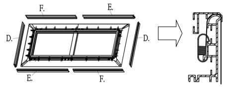
Connect edge trim frames (E/F) together using the *Center Joints- M4(a)* and secure with four of the *M4x4 Screws(m)* as show in *Step 1*. Repeat for other side.
