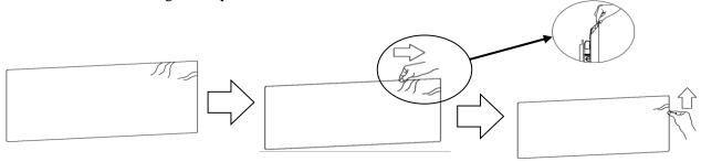
**Incorrect material installation** –The corners of the screen material are not properly wrapped along the edge of the frame leaving the material with unbalanced tension and an uneven finish. To correct, detach springs from material at the corner(s) where material does not lie flat along the edge of the frame, reposition the material so that it lies flat and wraps along the edge of the frame, and reattach springs to the material.
