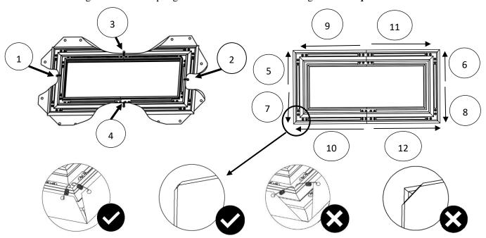
To avoid ripples forming in the material it is imperative that all of the corners are properly wrapped around the edges as illustrated in the check mark diagrams.
