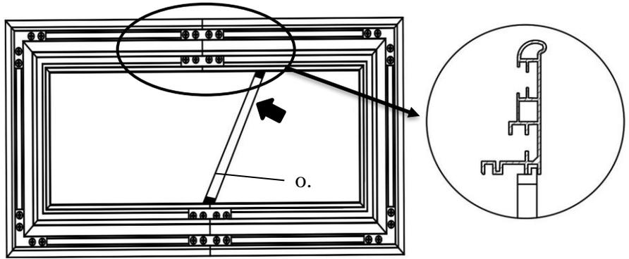
**Step 9:** Hook one end of the spring and secure inside the groove of the frame, use the *spring hook* (i) to attach the spring to the hole located on the screen material's outer edge in the following order.
