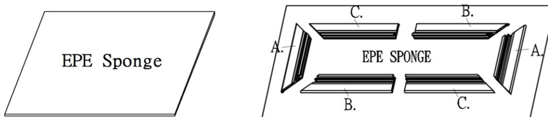
**Step 3:** Insert *center joint (a/b)* connectors into *one-half of the horizontal frame (B/C)* and secure with the *M4x7 screws (g)* as shown in the illustration below.
