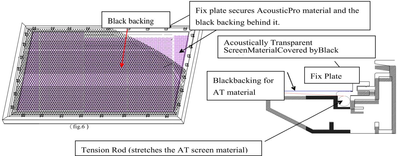
After the material has been installed, the backing will lie over the back of the white (AT) material and then be held into place by the fix plates as they are added (Fig.1-3). Interval markings reveal the best likely points of attachment (Fig. 1). The prongs on the fix plates (Fig. 2) straddle a lip on the back of the frame creating a friction hold that will firmly keep the material and backing in place (Fig. 3-4).
