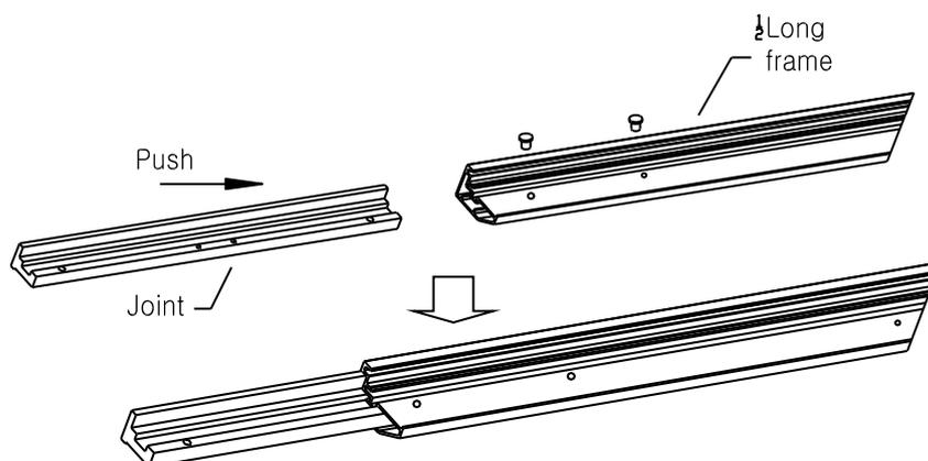
2. Insert the other horizontal frame piece to the **center joint** connector and then fasten it with 2 screws.
