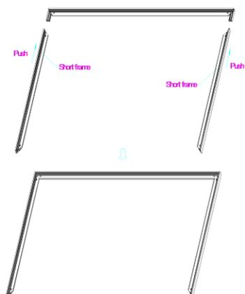
4. Join all four frame parts together following the steps showed below(**fig.2**).
