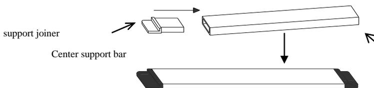
2. Insert the **Center Support Bar** into the upper top groove on the back of the frame (not where the fix plate inserts are) with the bottom end near the approximate center point of the frame and place it in at an angle so that both ends of the bar are in alignment with the groove (Fig. 8).
