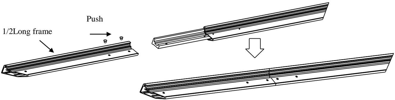
**Make sure the frame piece lines up correctly before you tighten the screws completely.**
