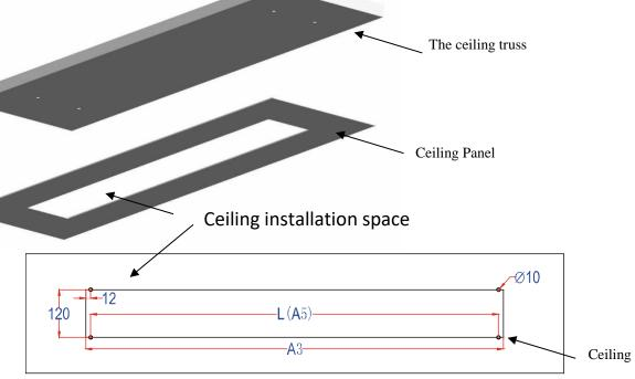
2. Drill 4 holes in the ceiling that correspond with the attachments on the various casing sizes.
