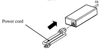
**Step 5.** Connect the LED Controller to the Power Supply
