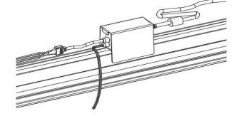
The controller will be hidden behind the screen. Make sure to have the receiver exposed below the frame as shown here.
