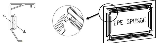
Step 5. Secure the elbow joints by fastening them with *M4x7 screws*(g), 4 at each corner.
