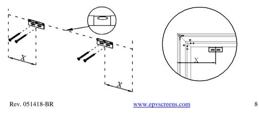
**Step 15**: Position the fixed frame screen onto the top wall brackets as shown below and push down at the center of the top of the frame to secure.
