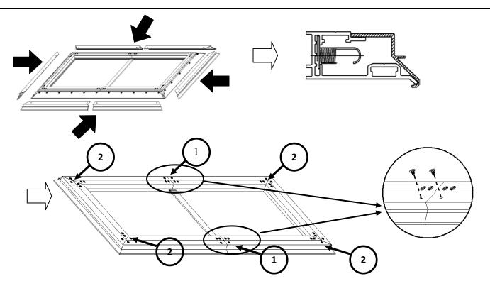
**Step 13**: Install the *angle cover (j)* on each corner of the frame and install the LED light strip to hold down the angle cover. Then insert the *LED light clip (l)* to hold the LED light strip in place.
