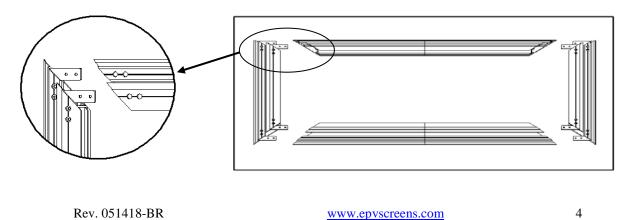
Step 6: Secure the elbow joints by fastening them with *M4x6 screws* (c), 4 at each corner.
