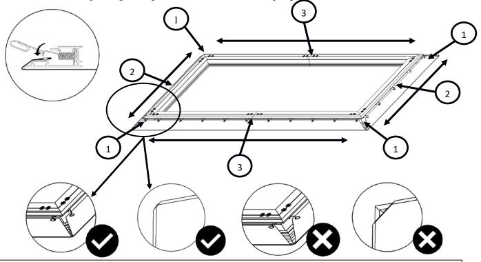
To avoid ripples forming in the material it is imperative that all of the corners are properly wrapped around the edges as illustrated in the check mark diagrams above.
