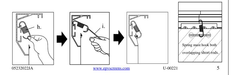
First connect on four corners, steps 1-4. make sure all four corners are fixed before proceeding with next spring.
