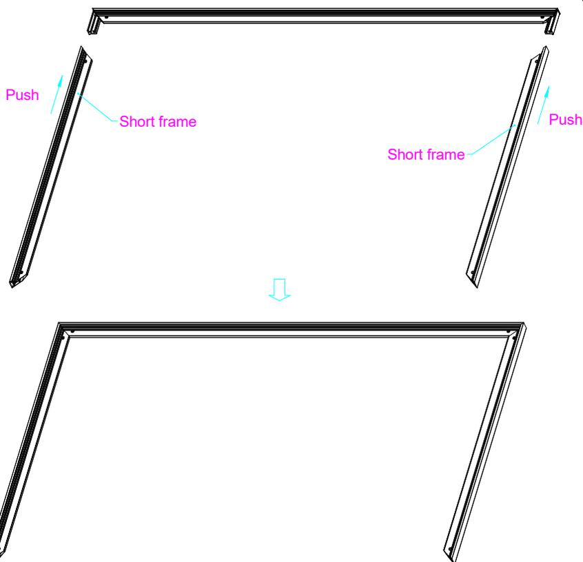
4. Join all four frame parts together following the steps showed below. After making sure that all four corners join at right angles to form a perfect rectangle, fasten the four angles together by using the (x8) joint screws included (**fig.2**).
