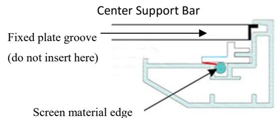
3. Slide the top end of the bar into the top center point location to complete center support bar installation. **This will provide added stability to your frame and added tension to the material.**
