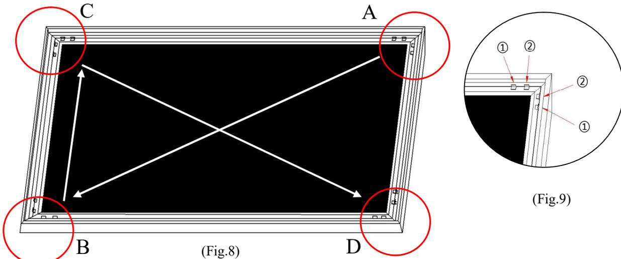
**Tip for attaching the last corner(D):**
