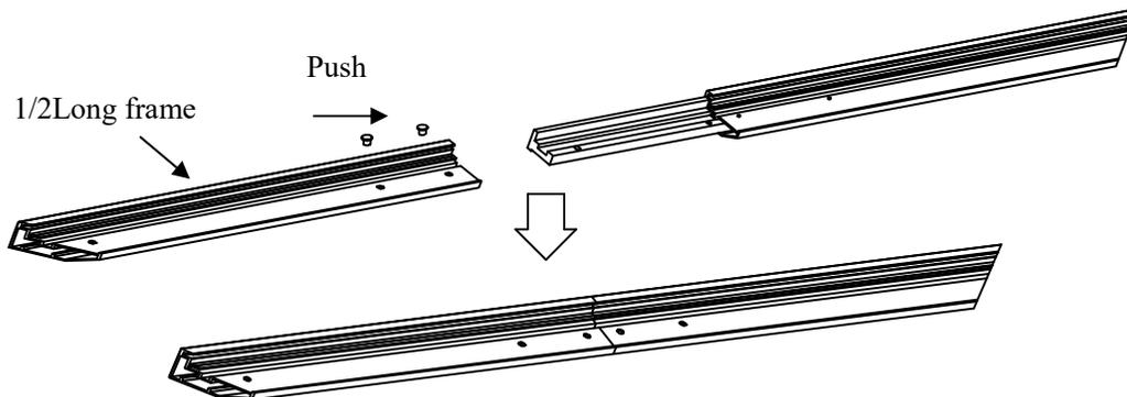
**Make sure the frame piece lines up correctly before you tighten the screws completely.**
