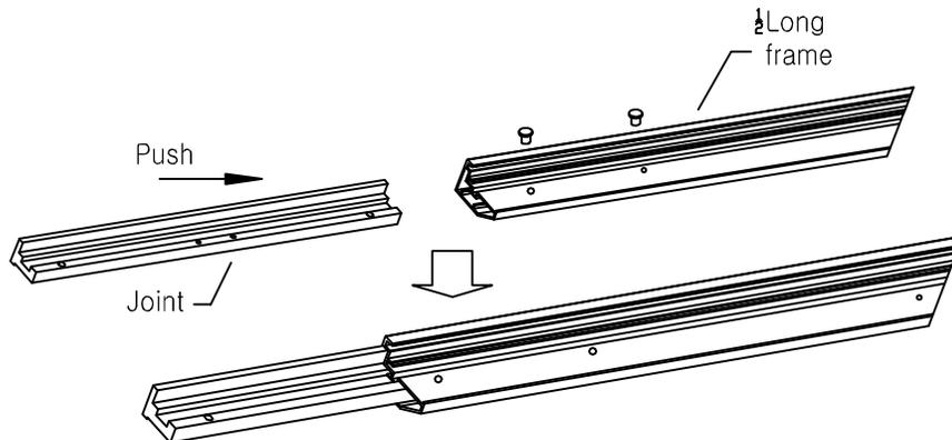
2. Insert the other horizontal frame piece to the **center joint** connector and then fasten it with 2 screws.
