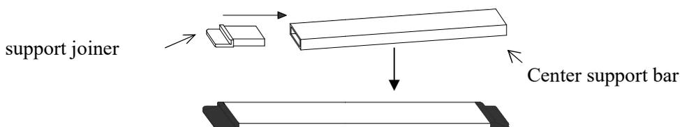
2. Insert the **Center Support Bar** into the upper top groove on the back of the frame (**not where the fix plate inserts**) with the bottom end near the approximate center point of the frame and place it in at an angle so that both ends of the bar are in alignment with the groove (Fig. 18 and 19).
