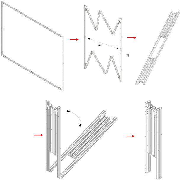
11. Store the screen in the provided *carrying bag* (*F*). Be sure to place folding frame, legs, and smaller parts into the carrying bag first and place the material on top to keep material from creasing or tearing.
