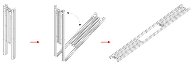
2. Next, unfold the horizontal sections by separating and pulling the left and right sides outwards.
