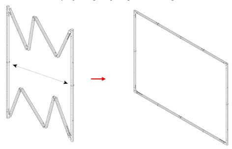
Note: When unfolding the frame and legs, be sure the latches on the hinges "click" into place. Please also make sure all 4 corners of the frame are at a  $90^{\circ}$  angle and the hinged support bar is straight and not bent.
